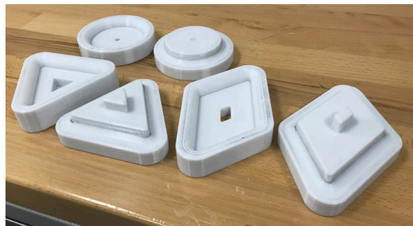
Figure 2-4: Custom flare tooling printed using polycarbonate.
