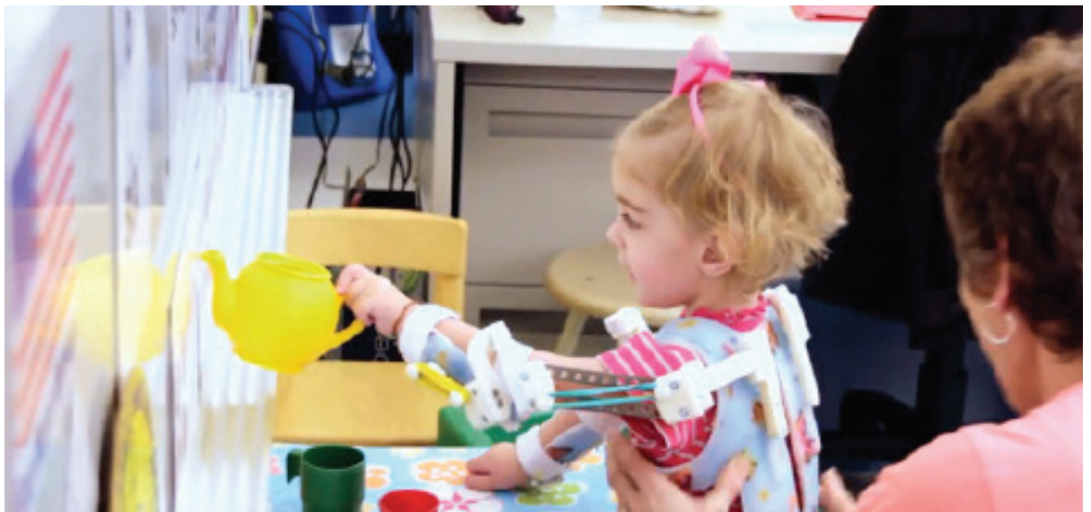
An FDM 3D printer allows Emma to wear a custom lightweight exoskeleton, which enables her to fully use her arms.
