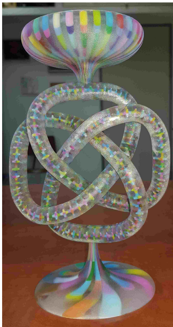
3D printed “chalice” model with colored microelements sliced by Voxel Print, and enclosed in translucent VeroClear™ material.
