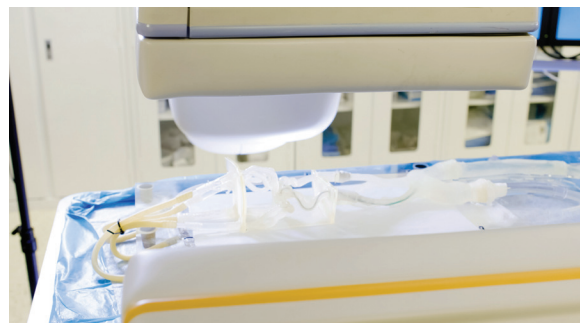
This 3D printed vascular testing model allows medical device designers and engineers to gather valuable performance feedback on device performance.
