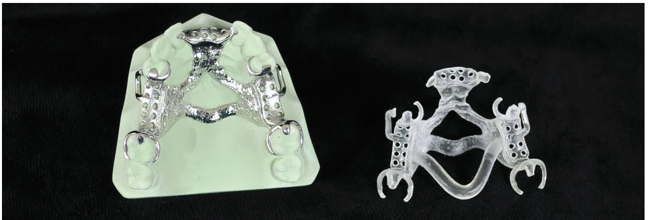
This cast frames, left, was created with the help of 3D printed biocompatible (MED610) material, right.
